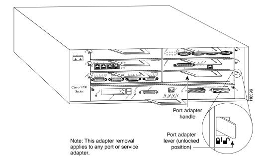
Step 3 Grasp the handle on the port adapter and pull the port adapter from the midplane, about halfway out of its slot. If you are removing a blank port adapter, pull the blank port adapter from the port adapter slot.
